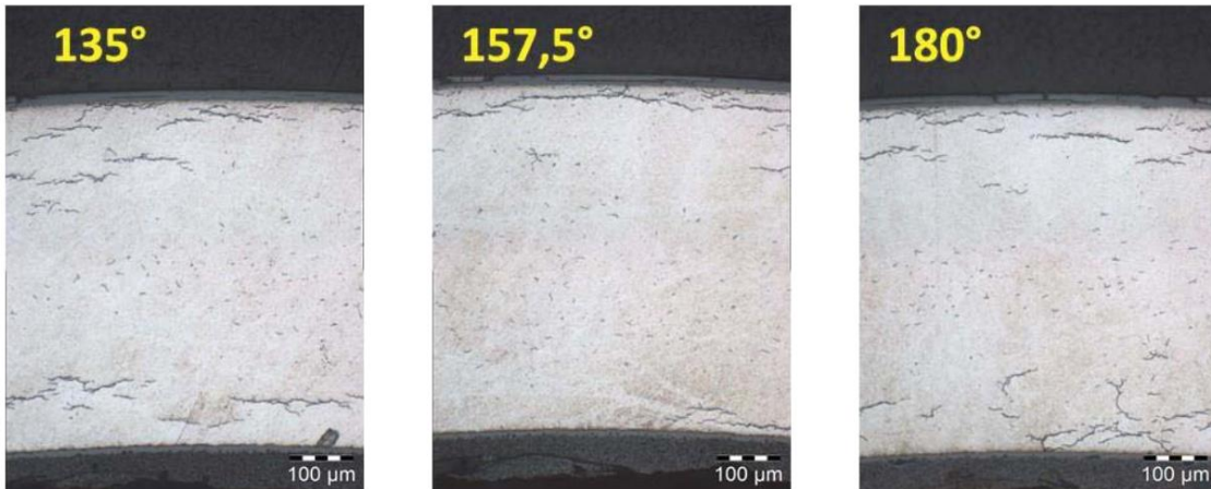
M5 Framatome irradiated 4 cycles in PWR, mean rod BU 63.7 GWd/t, span 8 (hottest localization)
